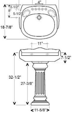
Dimensions of fixture are nominal and may vary within the range of tolerances established by ASMEI Standard A112.19.2-2018. Dimensions and specifications subject to change without notice.
